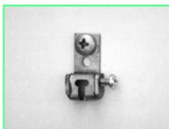
**Step 1:** Install two wall brackets using any type of wall fastener spaced the same distance as the hangers. Insert the self-tapping locking screws part way into the wall brackets.
